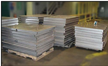
Featuring a heavy structural tube frame with 3" or 4" thick insulated floor panels, and leak-proof seal-welded construction.
